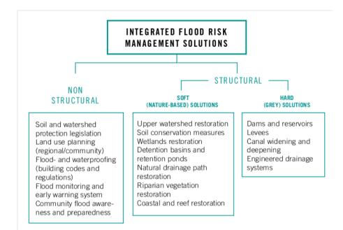
Figure 2 Structural and non-structural flood risk management solutions (adapted, source: Ilieva et al., 2018)
